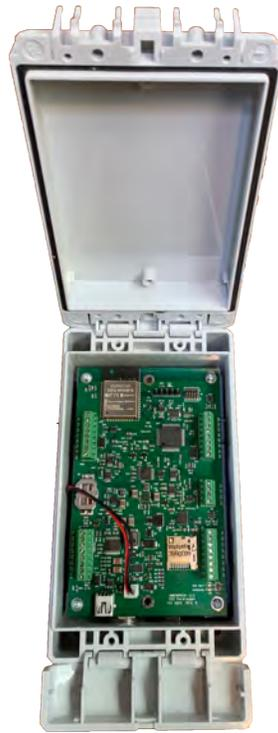
**Figure 1: Data Logger 222 with Integrated Battery Pack and Water-Tight Enclosure**
