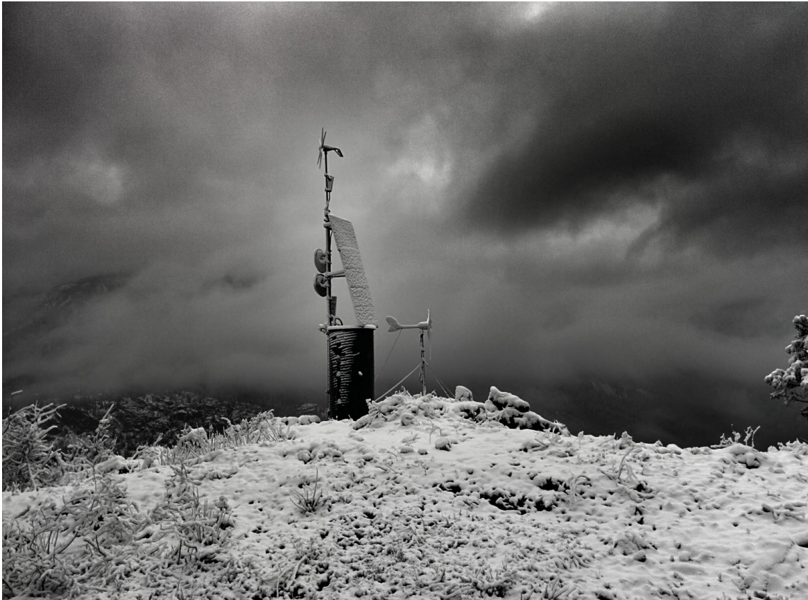
Figure 1- Example of remote off grid repeater site that will be monitored by the TriSonica Mini and Flex Q-Series SCADA equipment.
