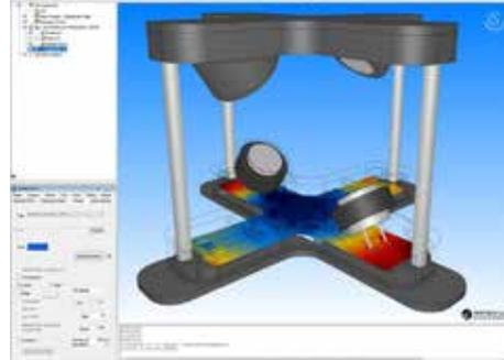
Figure 2: Thermal performance testing of the TriSonica Mini
