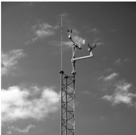
Figure 3: Tower with sensors installed measuring temperatures.
