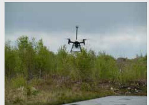
Figure 7: Capturing high resolution methane measurements from a UAS.
