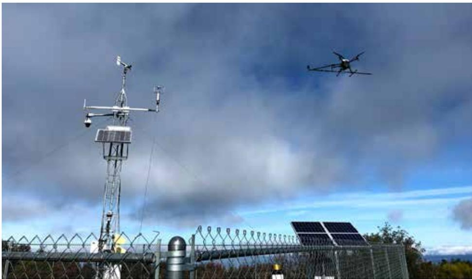
Figure 2: Calibration tests conducted with TriSonica Mini and RMY anemometer.
