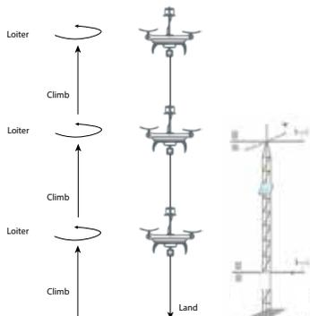
Figure 4: The climb and loiter approach used to capture atmospheric data.
