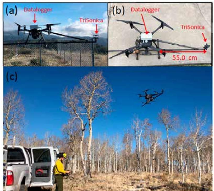
Figure 1: Photos of UAS system to showing system design and operation. (a) Horizontal view of system with hovering. (b) The TriSonica Mini is mounted on a carbon fiber pole extending 55.0 cm off the body of the UAS with the datalogger fixed to the top of the platform. (c) The profiling flight in the Fishlake National Forest, Utah, 7 November 2019.
