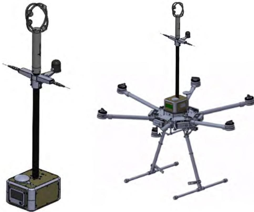
**Figure 2: TriSonica Sphere Integrated with BlueHalo's Atmospheric Characterization Payload (left); attached to a DJI Matrice 600 (right)**
